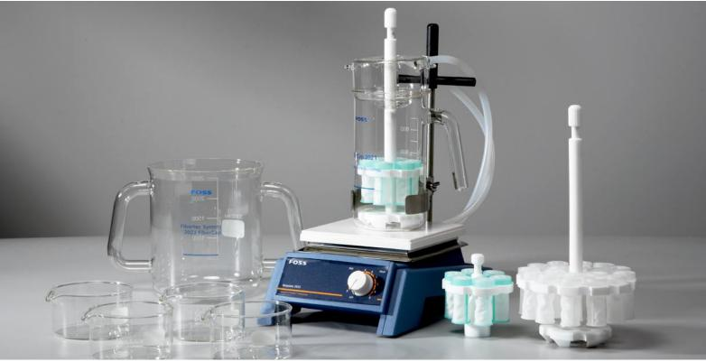
A modular system for simple analysis of crude and detergent fiber.
