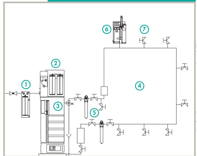
**A total water purification** system requires the main water purification system to be integrated into a centralized system. For example:
